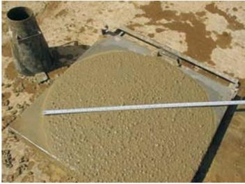
**Slump flow of 650mm for self-compacting G100 concrete**
