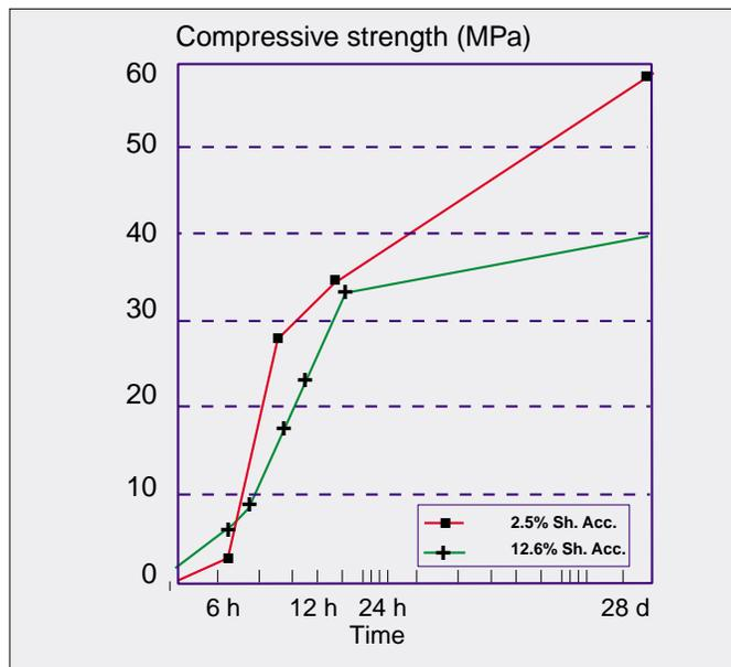
Figure 1 Strength development of shotcrete with accelerator
