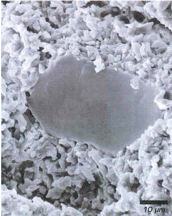
SEM image showing an alumina grain surrounded by a mullite network
