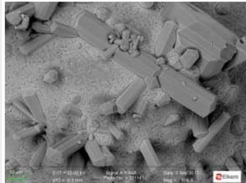
Examine growth of SiC (Carbide) and Si 3 N 4 (Nitride) crystals on a substrate
