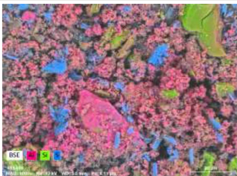
Mapping of Aluminium, Silicon and Sulphur in a crushed mineral
