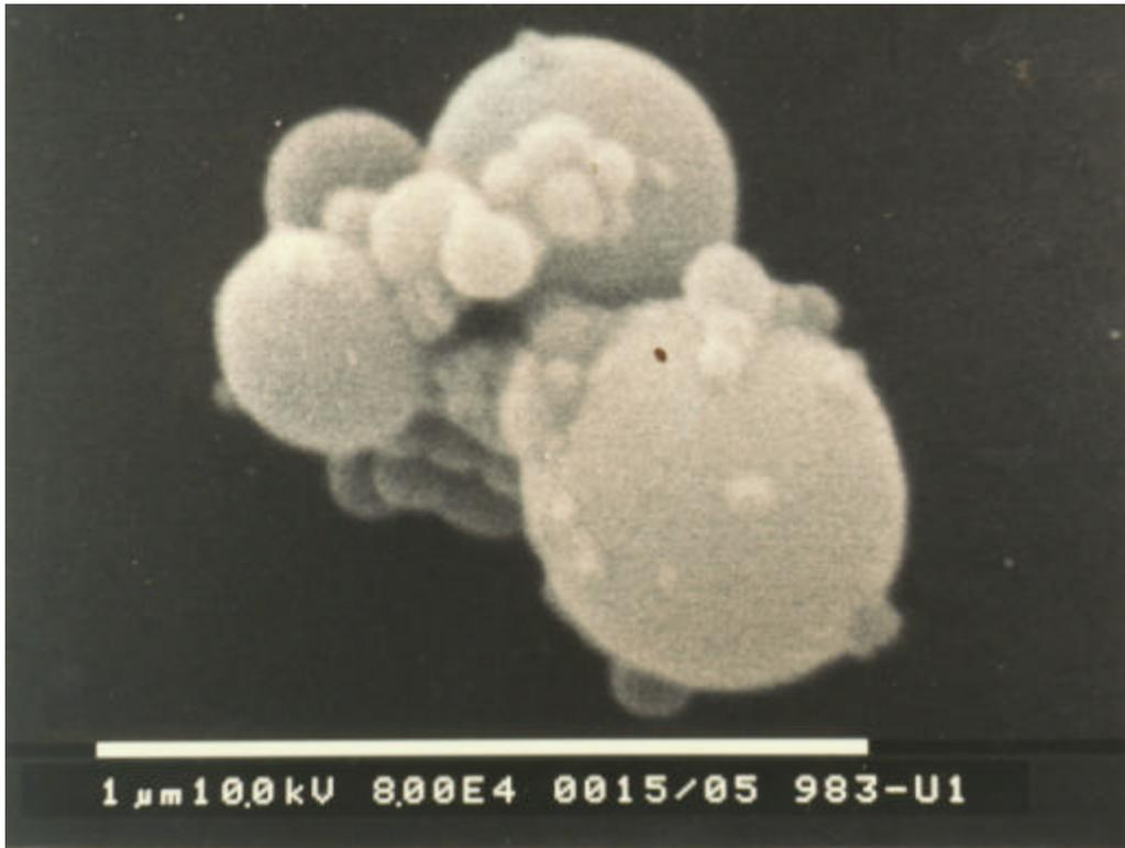
Figure 2: Micrograph of a microsilica cluster showing spherical appearance of the individual particles.
